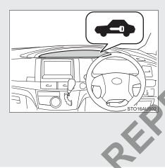
The indicator flashes after the "ENGINE START STOP" switch has been turned off to indicate that the system is operating.
