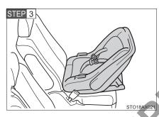
Place the child restraint system on the seat facing the rear of the vehicle.
