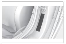
The tyre inflation pressure information is located on the body pillar of the driver's door.
