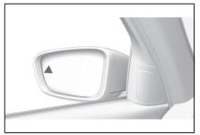
The warning light in the exterior mirror warns of a possible collision.
