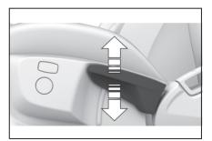
Pull the lever up or press the lever down repeatedly until the seat reaches the desired height.
