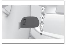
Press the lever upwards from the home position once, arrow 1.
