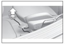
Pull the lever and slide the seat in the desired direction
