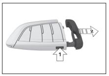
Press the button, arrow 1, and pull out the integrated key, arrow 2.
