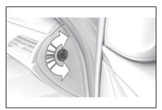
The key switch for front passenger airbags is located on the outside of the dashboard
