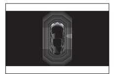
Obstacle markings are displayed at the sides of the vehicle to protect the vehicle's flanks
