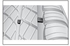
There are wear indicators from the tyre manufacturer distributed over the tyre circumference with a height of at least 1.6 mm, approx. 0.06 in, which serve as an indicator of tyre tread wear.
