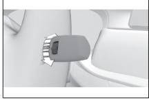
Turn the knurled wheel to set the sensitivity of the rain sensor.
