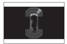
The approach of the vehicle to an object is shown on the Control Display. Objects that are further away are already displayed before an acoustic signal is given.
