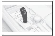
Press the selector lever out of selector lever position D to the left.
