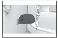
Press the lever upwards until the desired position is reached.
