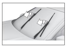
4 Press the button, arrow 1, and pull out wiper blade, arrow 2.
