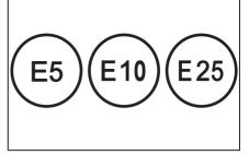
The engine has knock control. This means that different petrol grades can be used.
