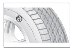
The tyres are identified on the tyre's side wall by RSC Runflat System Component.
