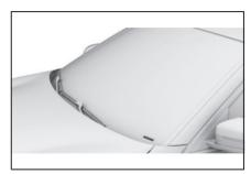
The vehicle identification number is additionally located behind the windscreen.
