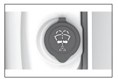
The reservoir for the washer fluid is located in the engine compartment.
