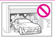
The exhaust includes colorless, odorless carbon monoxide (CO). Carbon monoxide (CO) can be inhaled without noticing and in the worst cases. can cause death. Make sure to not allow the engine to idle in a closed off garage or other location with poor ventilation
