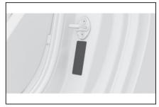
The vehicle identification number is on the type plate, on the left-hand side of the vehicle.
