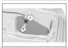
The on-board tool kit is located on the right in the boot, under a cover.
