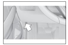
The OBD socket for checking emissions-relevant components is located on the driver's side.
