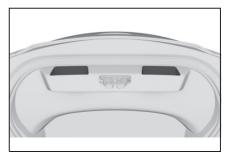
Pull the boot lid down using the handle recess.
