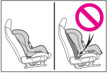
\*3: Use only a front-facing child restraint system when the airbag manual on-off switch is on.
