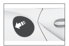
2 Turn the fuel tank cap anticlockwise.
