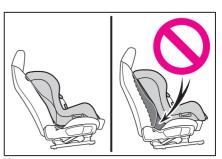
\*3: Use only a front-facing child restraint system when the airbag manual on-off switch is on.
