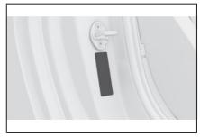
The vehicle identification number is on the type plate, on the right-hand side of the vehicle
