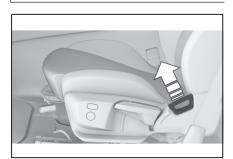
Pull the lever and apply your weight to or lift your weight off the backrest as required.
