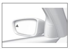
The warning light in the exterior mirror flashes if other vehicles are detected by the rear sensors when the vehicle is moving backwards.
