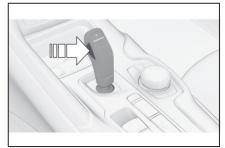
3 Briefly press the selector lever in the desired direction, possibly overcoming a resistance point. The selector lever returns to the middle position when released.
