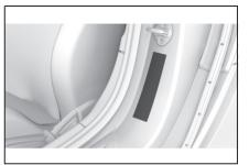
The tyre inflation pressure inscriptions can be found on the tyre pressure plate on the door pillar.
