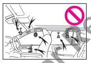
• Vehicles without smart entry & start system: Do not attach any heavy, sharp or hard objects such as keys and accessories to the key. The objects may restrict the SRS knee airbag inflation or be thrust into the driver's seat area by the force of the deploying airbag, thus causing a danger.
