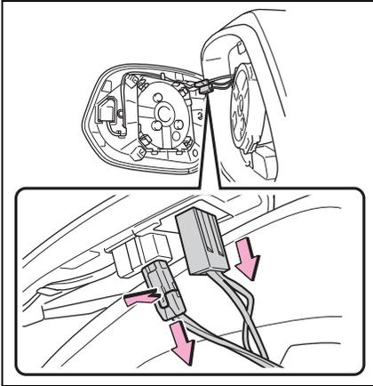
**3** Disconnect the tabs behind the mirror cover, and remove the mirror cover.
