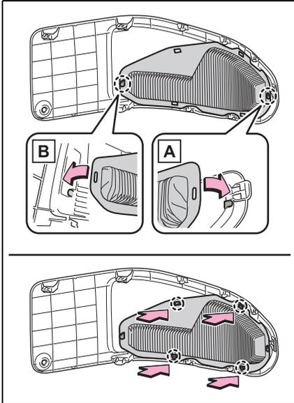
**8** Install the air intake vent cover.
