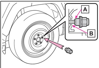
When replacing an aluminum wheel with an aluminum wheel, turn the wheel nuts until the washers **A** come into
