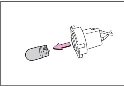
**8** Install a new light bulb then install the bulb base to the light unit by inserting it and turning the bulb base clockwise.
