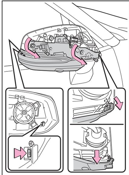
**6** Turn the bulb base counter-clockwise.
