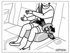
1. Sit the child on a junior (booster) seat. Run the lap and shoulder belt through or around the junior (booster) seat and across the child following the instructions provided by its manufacturer and insert the tab into the buckle taking care not to twist the belt.
