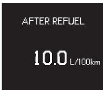
Displays the average fuel consumption since the vehicle was last refueled
