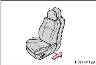
When you have to use a child restraint system, adjust the seat cushion to the fully rearward.
