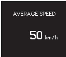
Displays the average vehicle speed since the engine was started or the function was reset
