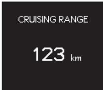
Displays the estimated maximum distance that can be driven with the quantity of fuel remaining
