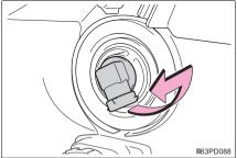
Replace the light bulb. Align the 3 tabs on the light bulb with the mounting, and insert.
