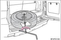
5 Pull out the spare tire and remove the holding bracket.
