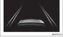
Indicates that the system is recognizing white (yellow) lines or a course\*. When the vehicle departs from its lane, the white line displayed on the side the vehicle departs from flashes orange.
