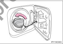
3 Hang the fuel tank cap on the back of the fuel filler door.
