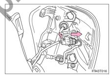
4 Rear turn signal light only: Unclip the connector wire.
