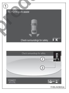
A simplified image is displayed on the upper corner of the screen when an obstacle is detected.
