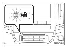
Close the doors and hood, and lock all the doors using the entry function (vehicles with smart entry & start system) or wireless remote control. The system will be set automatically after 30 seconds.
