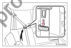
With center seat: Stow the center seat belt tabs in the cover set in the roof. (→P. 34)
