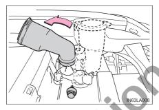
2 Unplug the connector while depressing the lock release.
