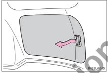
2 Unhook the strap and remove the tool bag.
