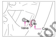
2 Bring the protruding part of the valve core tool into contact with the valve to discharge air.
