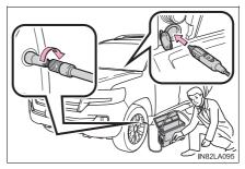
21 Read the inflation pressure on the pressure gauge.
