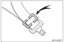
5 Latch the attaching clip of the upper anchorage strap onto the anchor fitting. (→P. 71)
