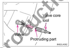
3 Pull out the valve core by turning it counterclockwise using the valve core tool.
