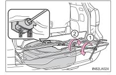
4 Lower the spare tire completely to the ground.
