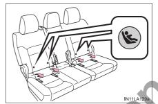
Check the positions of the exclusive fixing bars, and install the child restraint system to the seat.
