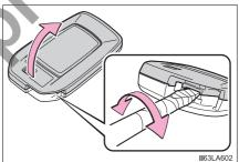
3 Remove the depleted battery.
