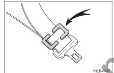
5 Latch the attaching clip of the upper anchorage strap onto the anchor fitting.  $(\rightarrow P. 71)$ Make sure the seat belt is tightly secured, and that there is not slack in the belt.
