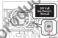
When the DPF system warning message goes out, the idling engine speed will have finished returning to normal.
