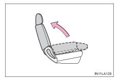
2 Take off the covers between the seat cushion and seatback, then confirm the position of the ISOFIX rigid anchors below the symbol in the seatback.
