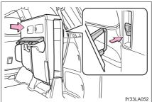
5 Remove the seat hook covers from the back of the seat cushion, and install them on the seat hooks.
