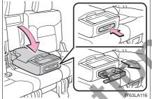
To open, pull down the armrest, press the button and release the rear cup holder on the armrest.
