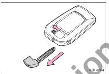
After using the mechanical key, store it in the electronic key. Carry the mechanical key together with the electronic key. If the electronic key battery is depleted or the entry function does not operate properly, you will need the mechanical key. ( $\rightarrow$ P. 632)
