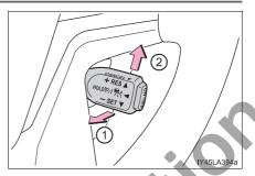
However, cruise control does not resume when the vehicle speed is approximately 40 km/h (25 mph) or less.
