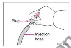
8 Connect the injection hose to the valve.
