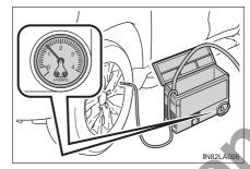
If the pressure is 130 kPa (1.3 kgf/cm<sup>2</sup> or bar, 18 psi) or above, fill the tire with air using the compressor until the specified inflation pressure is reached.
