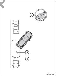
Leaving the vehicle stopped, turn the steering wheel all the way to the left.
