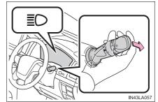
Press the Automatic High Beam switch.
