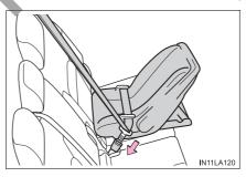
Install a locking clip near the tab of the lap and shoulder belt by inserting the lap and shoulder webbing through the recesses of the locking clip.
