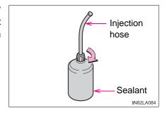
7 Remove the plug from the injection hose.
