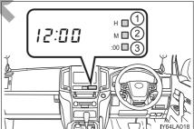
The clock can be adjusted by pressing the buttons.
