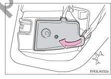
4 Unclip the connector wire and turn the bulb bases counterclockwise.
