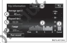
Average fuel consumption for the past 15 minutes is divided by color into past averages and averages attained since the engine switch was last turned to the "ON" position (vehicles without smart entry & start system) or IGNITION ON mode (vehicles with smart entry & start system). Use the displayed average fuel consumption as a reference.
