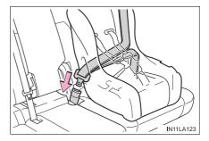
4 Install a locking clip near the tab of the lap and shoulder belt by inserting the lap and shoulder webbing through the recesses of the locking clip.
