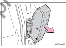
4 Unplug the connector while pressing the lock release.
