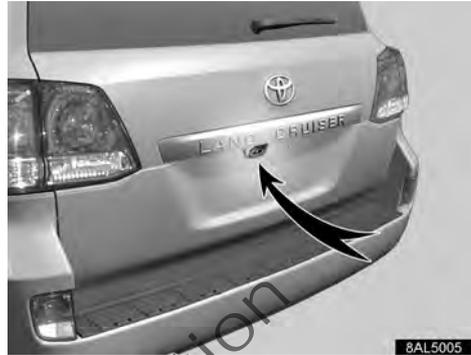
The parking assist system camera is located on the back door as shown in the illustration.
