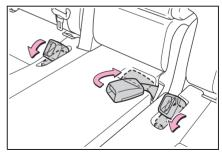
3 Pass the outer seat belts through the seat belt hangers and secure the seat belt plates.
