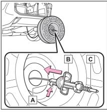
10 Tilt the holding bracket B so that it can easily be passed through the wheel opening.
