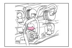
4 Turn the bulb base counterclockwise and remove it.
