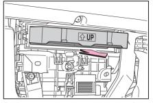
Remove the air conditioning filter from the filter case and replace it with a new one.
