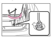
If the spare tire still cannot be lowered, the wire cable may be severed. Have the vehicle inspected by your Toyota dealer.
