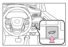
Opening the back door using the back door opener switch
