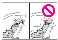
When installing a junior seat, if the child in your child restraint system is in a very upright position, adjust the seatback angle to the most comfortable position.
