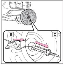
Fully depress the secondary latch A and install the bracket **B** to the hoist assembly **C**.
