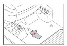
2 Remove the floor panel insulator pad.
