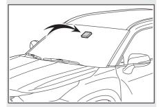
If the system judges that the vehicle is being driven over the speed limit, according to the recognized road signs, it notifies the driver through a visual notification and notification buzzer.
