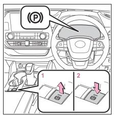
Pull the switch to set the parking brake
