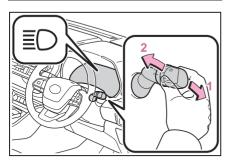
With the headlights on, push the lever away from you to turn on the high beams.
