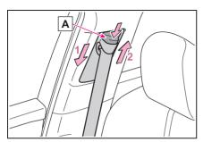
1 Push the seat belt shoulder anchor down while pressing the release button A. 2 Push the seat belt shoulder anchor up while pressing the release button A.
