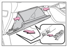
4 Unlock the filter cover (A), pull the filter cover out of the claws
