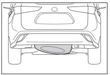
If the spare tire is slanted, the hoist assembly may be stuck in the wheel opening. If the spare tire rattles while driving, it may not be fully raised. Lower the spare tire to the ground and make sure that the hoist assembly is perpendicular to the wheel opening.
