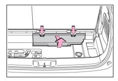
4 Remove the jack after removing the hook.
