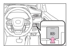
The Automatic High Beam indicator will come on when the system is operating.
