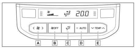
Adjust the rear seats fan speed setting
