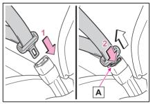
To fasten the seat belt, push the plate into the buckle until a click sound is heard.
