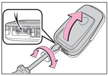
3 Remove the depleted battery.
