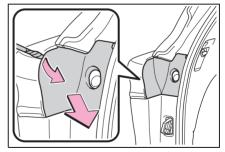
2 Remove the securing 2 screws and light unit.
