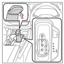
: While the engine switch is in ON and the brake pedal depressed\*, shift the shift lever while pushing the shift release button on the shift knob.
