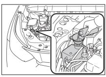
Start the engine and turn the air conditioning system on to check that the radiator cooling fan operates and to check for coolant leaks from the radiator or hoses
