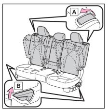
2 Pull the seatback folding lever to unlock the seatback. The seatback will be folded down
