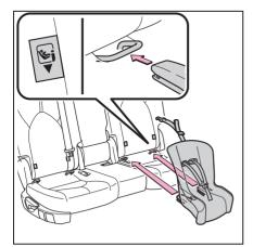
4 After installing the child restraint system, rock it back and forth to ensure that it is installed securely. (→P.50)
