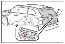
Opening/closing the back door using the power back door switch on the back door
