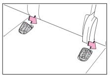
2 Pass the outer seat belts through the seat belt hangers and secure the seat belt plates.
