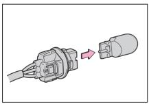
3 Install a new light bulb, and then install the bulb base to the light unit by inserting it and turning the bulb base clockwise.
