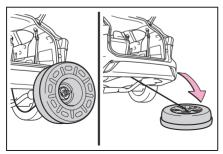
6 Before raising the tire, make sure that the hoist assembly is perpendicular to the wheel opening. (Try to place the tire directly beneath the vehicle, near where the wire cable is hanging from.)
