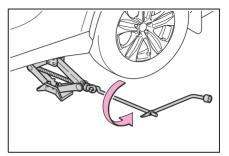
**4** Securely tighten the wheel nuts two or three times in the order
