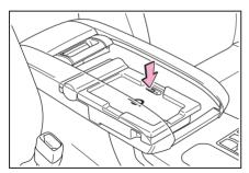
3 Place a portable device on the charging area with its charging surface facing down. Depending on the portable device, its charging coil may not be in the center of the device. In this case, place the portable device so that its charging coil is centered in the charging area.
