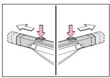
3 To install the luggage cover unit, with the lock release buttons facing upward, insert one end into the recess, then compress the other end and insert it into the other recess
