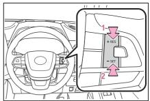
1 Increases the speed (Except when the vehicle has been stopped by system control in vehicle-to-vehicle distance control mode)
