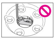
Do not attempt to turn the spare tire clamp bolt without a tire on the hoist assembly, as doing so may cause the wire cable to slip off of the shaft inside the unit and the wire cable may not be able to be raised or lowered. If the spare tire clamp bolt has been turned without a tire on the hoist assembly and the wire cable cannot be raised or lowered, contact your Toyota dealer.
