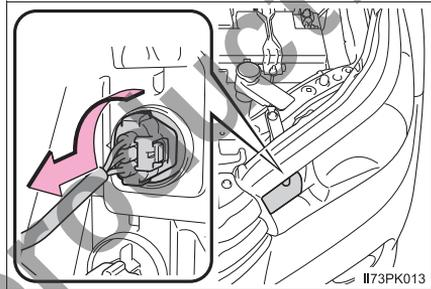
**2** Remove the light bulb.
