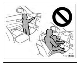
Do not hold a child on your lap or in your arms. Use a child restraint system in the rear seat. For instructions concerning the installation of a child restraint system, see "Child restraint" on page 53.
