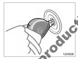
The engine immobilizer system is a theft prevention system. When you insert the key in the engine switch, the transponder chip in the key's head transmits an electronic code to the vehicle. The engine will start only when the electronic code in the chip corresponds to the registered ID code for the vehicle.
