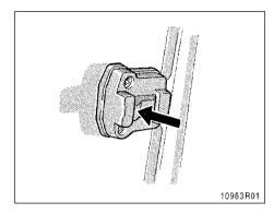
Push the lever to unlock and slide the window.
