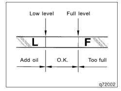
With the engine at operating temperature and turned off, check the oil level on the dipstick.
