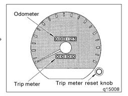
The odometer records the total distance the vehicle has been driven. The trip meter may be set to zero to record the distance on each trip. To reset the trip meter, press the trip meter reset knob.
