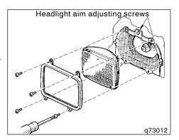
3. Loosen the retainer screws and take out the beam unit together with the retainer, unplugging the connector. Remove the rubber cover.
