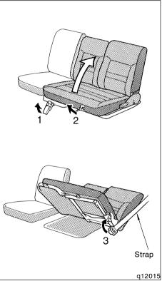
To open the engine access hold cover, release the latch and push the lock release lever sideward. Then raise the engine access hole cover with the seatbacks in the normal upright position. After lifting the cover up, hold it open with the strap.
