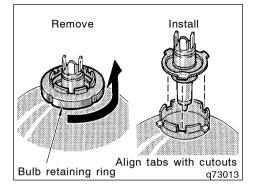
4. Remove the bulb retaining ring and bulb. Install a new bulb and the bulb retaining ring.
