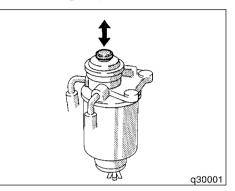
If you run out of fuel and the engine dies, the engine may not restart after refueling. In such case, operate the priming pump until you feel more resistance.
