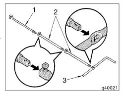
Put the jack handle, jack handle extensions and jack handle end together as shown in the illustration.
