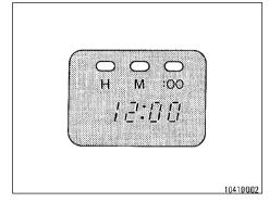
The digital clock indicates the time with the ignition key at the "ACC" or "ON" position. To reset the hour, depress the "H" button. To reset the minutes, depress the "M" button. To adjust the time to a full hour, depress the ":00" button.
