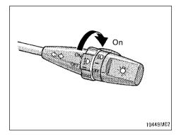
To turn on the front fog lights, twist the band of the headlight and turn signal switch lever. They will come on when the tail lights are turned on.
