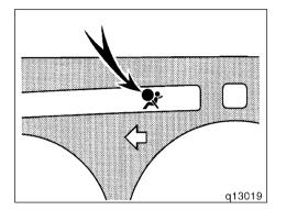
This indicator comes on when the ignition key is turned to the "ACC" or "ON" position. It goes off after about 6 seconds. This means the SRS airbag is operating properly.
