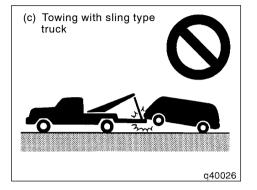
(c) Towing with sling type truck
