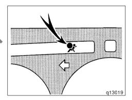
This SRS airbag system has a service reminder indicator to inform the driver of operating problems. If either of the following conditions occurs, this indicates a malfunction of the airbag. Contact your Toyota dealer as soon as possible to service the vehicle.
