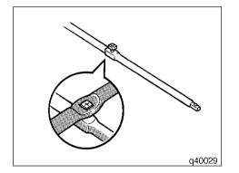
When connecting the jack handle extension/extensions and jack handle end, use the jack handle to tighten the bolt on the joint as shown in the illustration.
