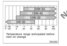
If you use SAE 10W-30 or a higher viscosity engine oil in extremely low temperatures, the engine may become difficult to start, so SAE 5W-30 engine oil is recommended.
