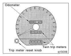
The odometer records the total distance the vehicle has been driven. The twin trip meters may be set to zero to record two different distances independently. To reset the upper trip meter, press the trip meter reset knob. To reset the lower meter, turn the knob clockwise and press it.
