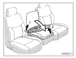
To use the center console box, pull the lever up and tilt the center seatback forward until it locks.
