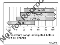
If you use SAE 10W-30 or a higher viscosity engine oil in extremely low temperatures, the engine may become difficult to start, so SAE 5W-30 engine oil is recommended.
