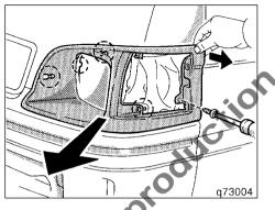
2. Remove the headlight door retaining screw and puil out the headlight door.
