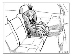
• A forward-facing child restraint system should be allowed to be installed on the front passenger seat only when it is unavoidable.
