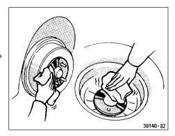
Before putting on wheels, remove any corrosion on the mounting surfaces with a wire brush or such. Installation of wheels without good metal-to-metal contact at the mounting surface can cause wheel nuts to loosen and eventually cause a wheel to come off while driving.
