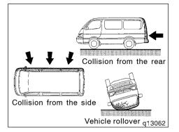
The SRS airbag is not designed to inflate if the vehicle is involved in a side or rear collision, if it rolls over, or if it is involved in a low-speed frontal collision.
