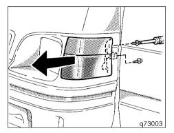
1. Open the front door. Remove the parking, front turn signal and side turn signal light retaining screws and take out the light unit. Then unplug the connectors.
