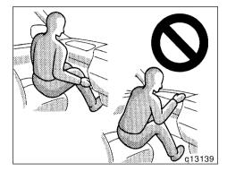
• Do not sit on the edge of the seat or lean over the dashboard when the vehicle is in use, since the front airbags inflate with considerable speed and force. Otherwise, you may be killed or seriously injured. Sit up straight and well back in the seat, and always use your seat belt properly.
