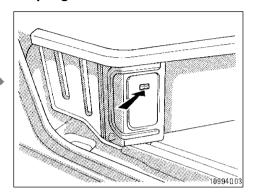
To turn on the rear interior lights, push the switch in
