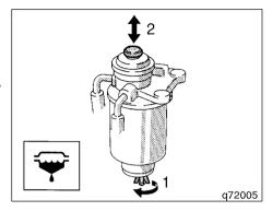
When the fuel filter warning light comes on, the water in the fuel filter must be drained immediately.
