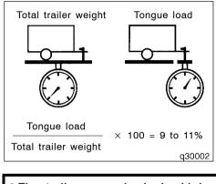
• The trailer cargo load should be distributed so that the tongue load is 9 to 11% of the total trailer weight, not exceeding 140 kg (308 lb.).
