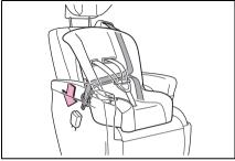
6 If your child restraint system is not equipped with a lock-off (a seat belt locking feature), secure the child restraint system using a locking clip.
