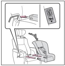
5 After installing the child restraint system, rock it back and forth to ensure that it is installed securely. (→P.81)
