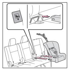
4 After installing the child restraint system, rock it back and forth to ensure that it is installed securely. (→P.64)
