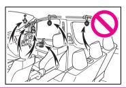
Wagon\*: Do not attach anything to areas such as a door, windshield, side windows, front or rear pillar, roof side rail and assist grip.
