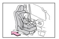
Do not allow the child to lean his/her head or any part of his/her body against the door or the area of the seat, front or rear pillars, or roof side rails from which the SRS side airbags or SRS curtain shield airbags deploy even if the child is seated in the child restraint system. It is dangerous if the SRS side airbags and curtain shield airbags inflate, and the impact could cause death or serious injury to the child.
