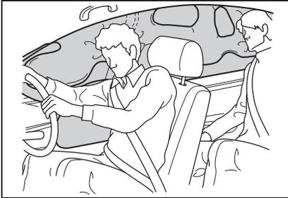
The driver's and front passenger's SRS side airbags and SRS curtain shield airbags deploy independently of each other since each has its own impact sensor. Therefore, they may not both deploy in the same accident. Also, the SRS side airbag and SRS curtain shield airbag deploy independently of the driver's and front passenger's SRS frontal airbags in the steering wheel and instrument panel.
