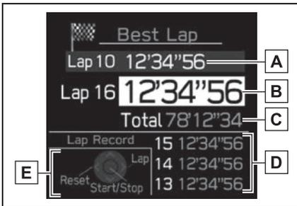
**A** Fastest lap time (measurement screen)
