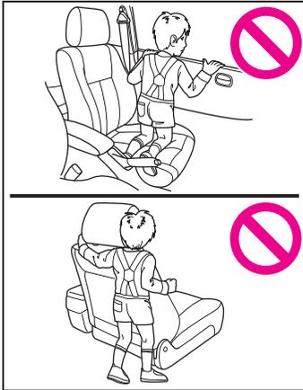
In the event of an accident, the force of SRS side airbag and/or SRS curtain shield airbag deployment could injure the child seriously because his/her head, arms or other parts of the body are too close to the SRS side airbag and/or SRS curtain shield airbag.
