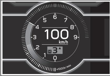
The engine speed at which the REV indicator is displayed can be changed on
