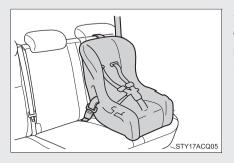
Seat belts equipped with a child restraint locking mechanism (ALR/ELR belts on the rear seats) (→P. 55)
