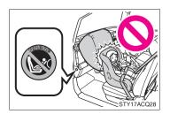
Extreme Hazard! Do not use a rearward facing child restraint on a seat protected by an airbag in front of it! This is because the force of the rapid inflation of the front passenger airbag can cause death or serious injury to the child.
