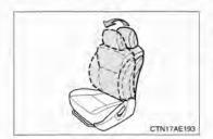
When you have to use a child restraint system in the front passenger seat, adjust the seatback to the most upright position.
