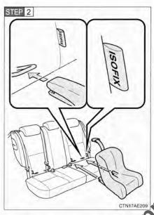
Check the positions of the exclusive fixing bars, and install the child restraint system to the seat.
