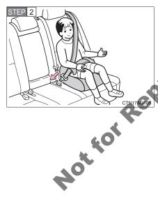
Sit the child in the junior seat (booster seat). Fit the seat belt to the junior seat (booster seat) according to the manufacturer's instructions and insert the plate into the buckle. Make sure that the belt is not twisted.
