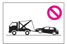
Towing with a wheel-lift type truck
