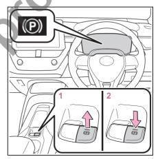
1 Pull the switch to set the parking brake
