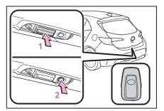
1 Press the button to unlock the back door.
