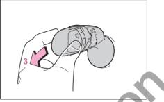
3 Washer/wiper dual operation The wiper will automatically operate a couple of times after the washer squirts.
