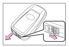
To prevent damage to the key, cover the tip of the flathead screwdriver with a rag.
