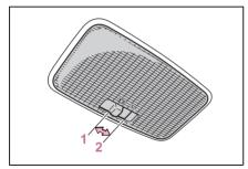
1 Turns the door position on The rear interior light turns on/off together the front interior lights. When a door is opened while the front and rear interior light door position is on, the lights turn on.
