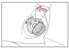
4 Vehicles with a smart entry & start system: To stop the engine, press and hold the engine switch for 3 consecutive seconds or more, or press it briefly 3 times or more in succession.
