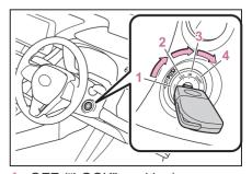
**1** OFF ("LOCK" position) The steering wheel is locked and the key can be removed. (vehicles with a continuously variable transmission: The key can be removed only when the shift lever is in P.)
