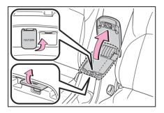
The power outlet can be used when The engine switch is in ACC or ON.
