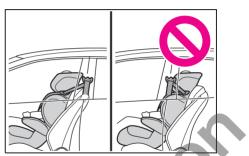
When installing a junior seat, if the child in your child restraint system is in a very upright position, adjust the seatback angle to the most comfortable position. And if the seat belt shoulder anchor is ahead of the child seat belt guide, move the seat cushion forward.
