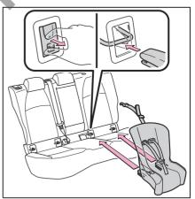
3 After installing the child restraint system, rock it back and forth to ensure that it is installed securely. (→P.44) 1
