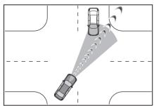
When turning left/right and an oncoming pedestrian or bicycle is detected
