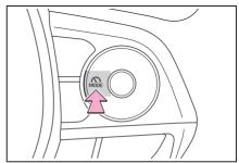
2 Using the accelerator pedal, accelerate or decelerate to the desired vehicle speed (approximately 30 km/h [20 mph] or more), and press the driving assist switch to set the set vehicle speed.
