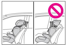
When installing a junior seat, if the child in your child restraint system is in a very upright position, adjust the seatback angle to the most comfortable position.
