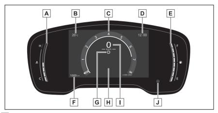
A Engine coolant temperature gauge
