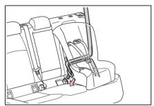
4 If your child restraint system is not equipped with a lock-off (a seat belt locking feature), secure the child restraint system using a locking clip.
