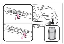
Press the button to unlock the back door.
