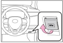
2 Pull the auxiliary catch lever to the left and lift the hood
