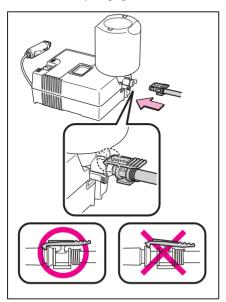
**5** Remove the valve cap from the valve of the punctured tire.
