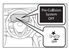
The pre-collision setting can be changed on the customize settinas. (→P.377)
