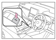
Each time the switch is pressed, the system changes between power mode and normal mode.
