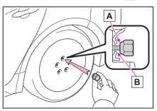
When replacing an aluminum wheel with a steel wheel (including a compact spare tire), tighten the wheel nuts until the tapered portion A comes into loose contact with the disc wheel seat
