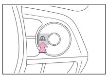
2 Using the accelerator pedal, accelerate to the desired vehicle speed (approximately 30 km/h [20 mph] or more), and press the driving assist switch to set the set vehicle speed.
