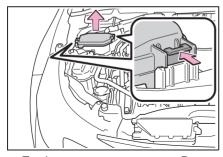
► Engine compartment: type B fuse box
