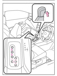
→: While the engine switch is in ON and the brake pedal depressed<sup>\*</sup>, shift the shift lever while pushing the shift release button on the shift knob.
