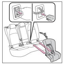
3 After installing the child restraint system, rock it back and forth to ensure that it is installed securely. (→P.50)
