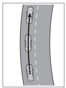
• When the function is operating, if the vehicle is likely to depart from its lane, the driver will be alerted via a display and buzzer.
