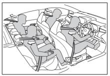
The pretensioners help the seat belts to quickly restrain the occupants by retracting the seat belts when the vehicle is subjected to certain types of severe frontal or side collision
