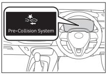
If the system determines that the accelerator pedal is strongly depressed, the following icon and message will be displayed on the multi-information display.
