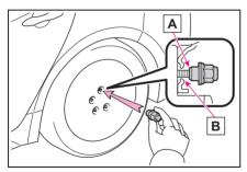
When replacing an aluminum wheel with an aluminum wheel, turn the wheel nuts until the washers **A** come into loose contact with the disc wheel **B**.
