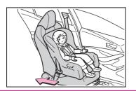
Do not allow the child to lean his/her head or any part of his/her body against the door or the area of the seat, front or rear pillars, or roof side rails from which the SRS side airbags or SRS curtain shield airbags deploy even if the child is seated in the child restraint system. It is dangerous if the SRS side and curtain shield airbags inflate, and the impact could cause death or serious injury to the child.
