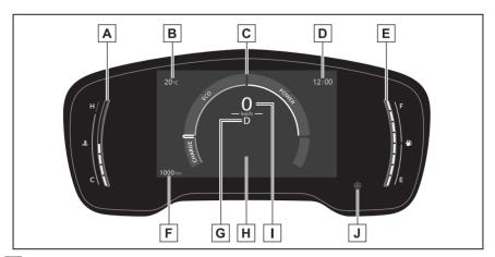
A Engine coolant temperature gauge
