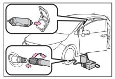
21 Turn the compressor switch on and wait for several seconds, then turn it off. Check the tire inflation pressure.
