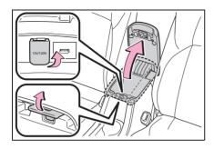
■ The power outlet can be used when The power switch is in ACC or ON.
