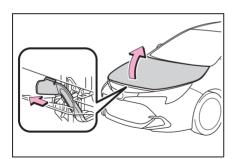
**3** Hold the hood open by inserting the support rod into the slot.
