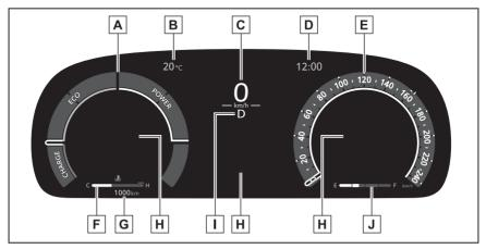
A Hybrid System Indicator/Tachometer
