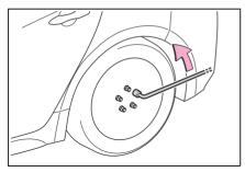
4 Turn the tire jack portion A by hand until the center of the recessed portion of the jack is in contact with the center of the jack point.
