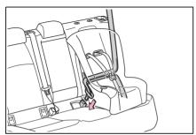
4 If your child restraint system is not equipped with a lock-off (a seat belt locking feature), secure the child restraint system using a locking clip.
