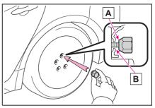
When replacing an aluminum wheel with a steel wheel, tighten the wheel nuts until the tapered portion A comes into loose contact with the disc wheel seat B.
