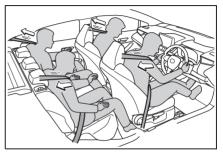
The pretensioners help the seat belts to quickly restrain the occupants by retracting the seat belts when the vehicle is subjected to certain types of severe frontal or side collision
