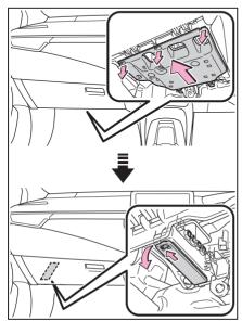
3 Remove the fuse with the pullout tool.
