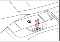
Place a portable device on the charging tray.
