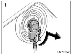
1. Open the bonnet. Turn the bulb base counterclockwise to the front of the vehicle as shown.
